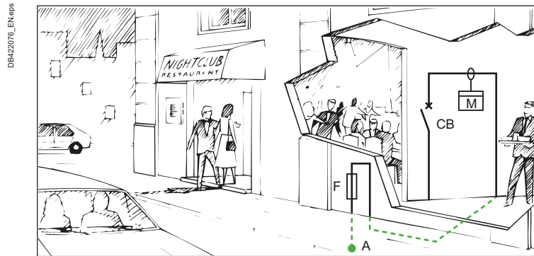
The service cable terminates in a flushmounted wall cabinet which contains the isolating fuse links, accessible from the public way. This method is preferred for esthetic reasons, when the consumer can provide a suitable metering and main-switch location.
