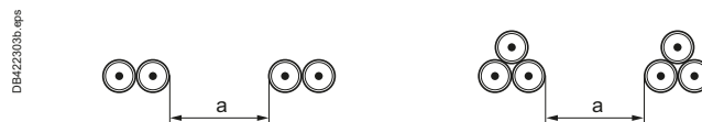
Fig. G18 Reduction factors for more than one circuit, single-core or multi-core cables laid directly in the ground. Installation method D. (table B.52.18 of IEC 60364-5-52)
